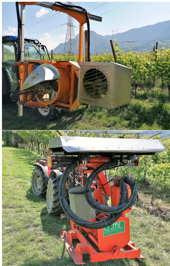
Figure 3.5: Pictures of the Machines used for defoliation
