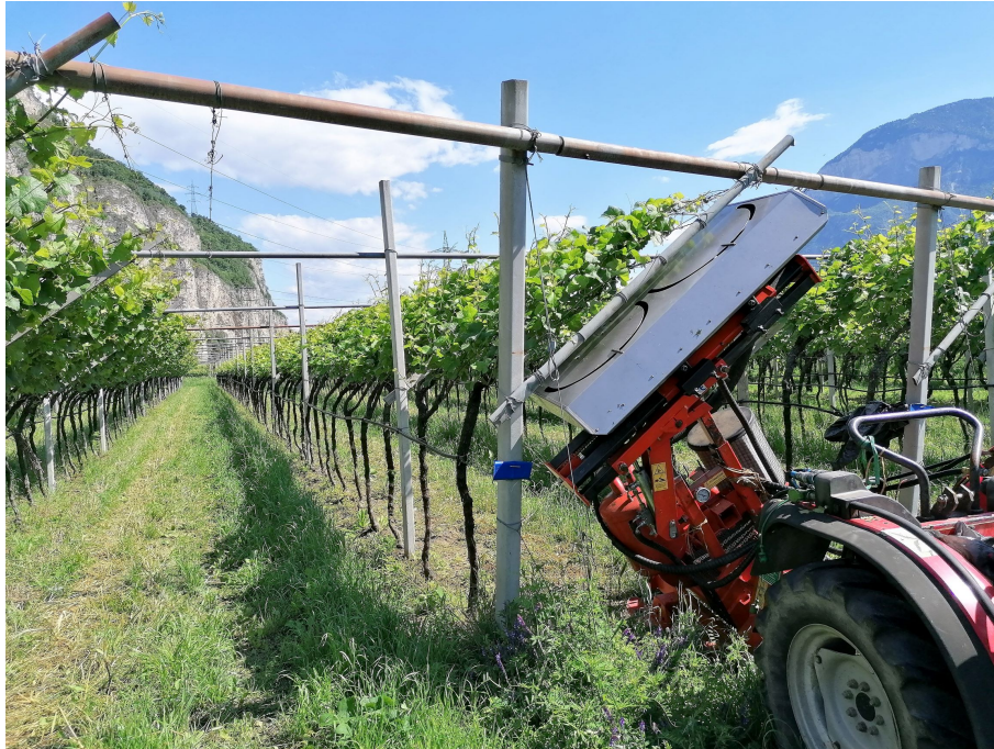
Figure 2.4: A pneumatic leaf removal machine being used on a pergola training system
