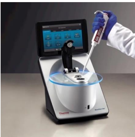
Figura 6: Thermo Scientific™ NanoDrop™ One.
